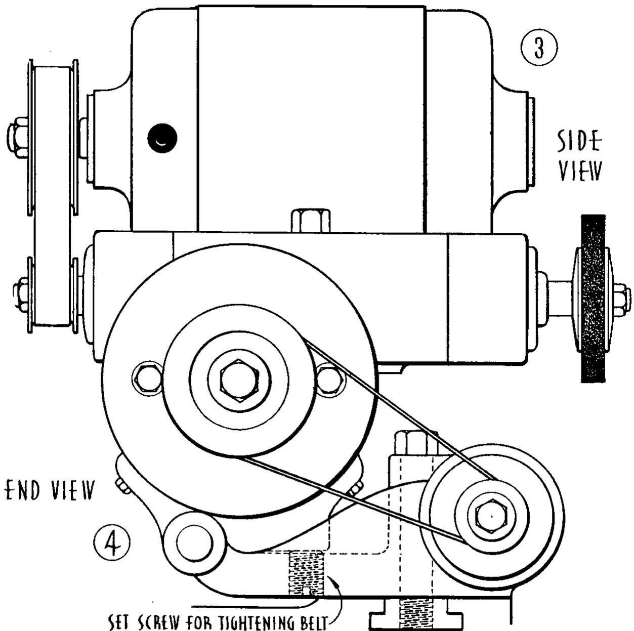
Ball bearing, mountable directly on the slide rest of the lathe, this very good grinder will enable you to turn out fine surfaces.
