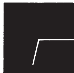
Diode in series with 51Ω
