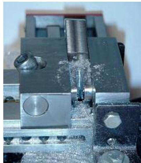
A 19-mm long piece of 14-mm diameter steel rod was drilled through with a 8 mm drill. Then sawn in two lengthwise, and used as top and bottom segment for the pressure screw. The 8 mm hole in the bottom segment was milled oval.
