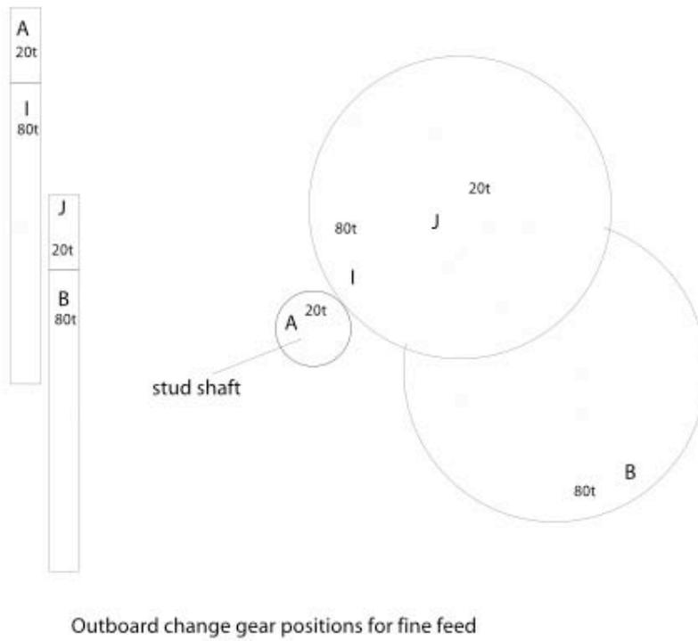
**Figure 11: Outboard change gear positions for fine feed**
