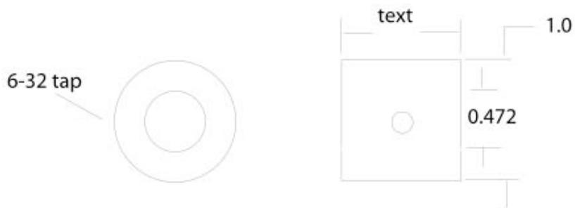
**Figure 6: "D" gear end fillers**
