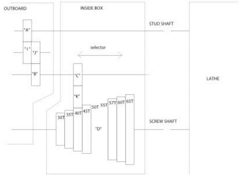
"A" is stud gear and can be changed
