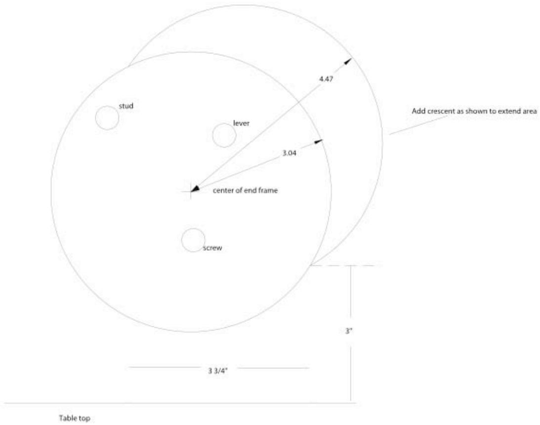
**Figure 12: End frame modification**
