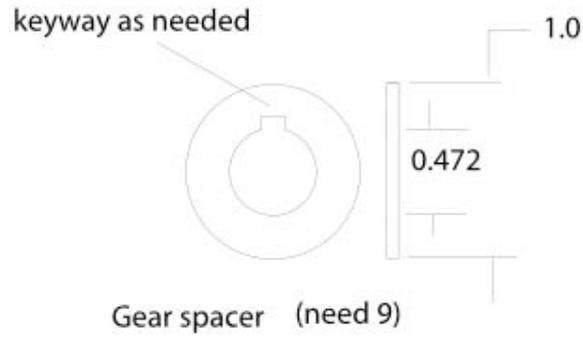
**Figure 5: Gear spacer**
